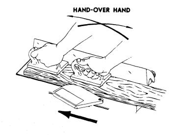
This means that once the work piece has passed the cutter head onto outfeed table, one hold down/push block must always maintain contact with the work piece with outfeed table.
